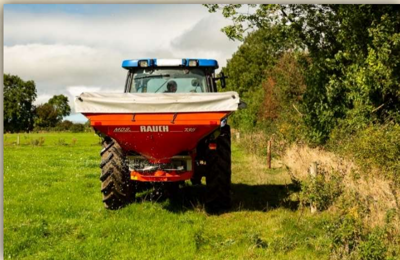
Fertiliser spreader disc shut off on the hedgerow side prevents nutrients reaching the field margin
